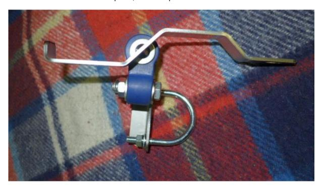
Below you see an example of a self-made bracket with rubber dampers:
